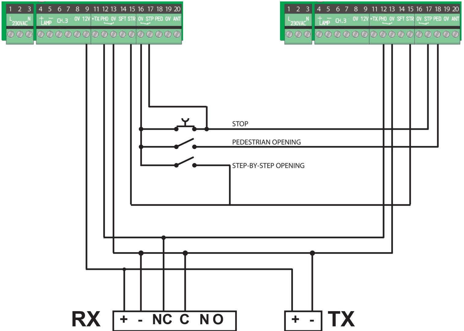
This configuration is necessary to link the commands by cable and the photocells. It is necessary an external receiver to unify the commands by radio (otherwise with a classic programming procedure, one central could receive the signal before than the other one, and cause a wrong functioning).
